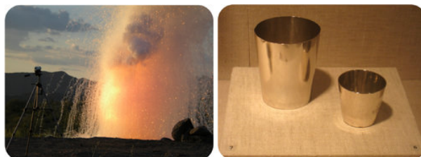
Figure 16.5.1: On the left, sodium reacts with water. On the right, silver in the form of cups do not react with water.
